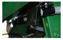
An 18-outet deflector package includes deflectors and angle iron mounting straps to
