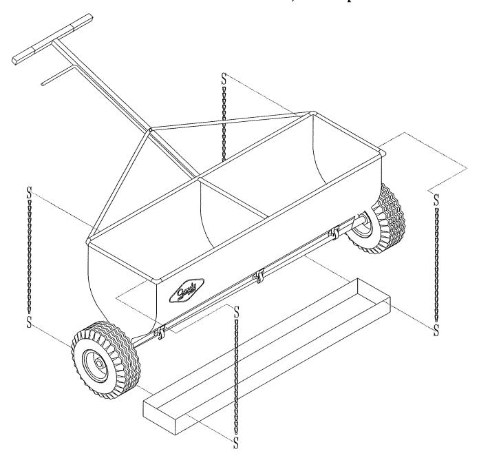
Attach calibration pans with chain, wire or appropriate suspender to be provided by customer.
