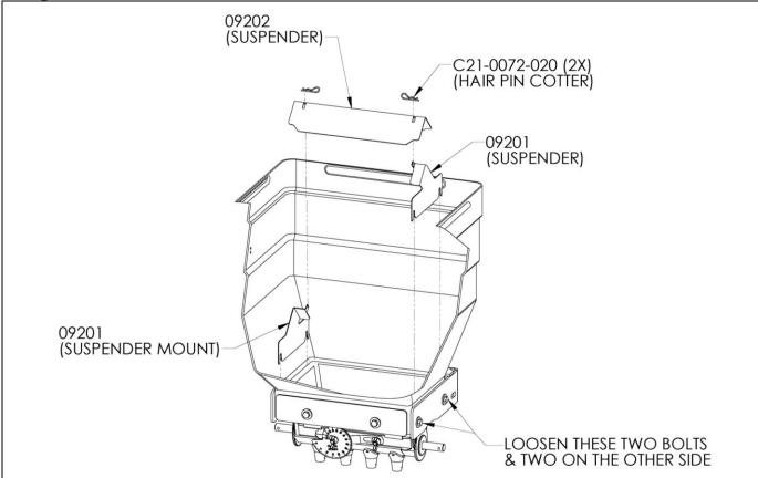
Loosen the bolts shown in diagram above. Locate suspender mounts (09201) and push insert mount down between hopper and bottom insert (silver in color) until it bottoms out on the two bolts that were loosened. Repeat for other mount. Tighten the two bolts on each side securely. Place suspender plate (09202) on top of the mounts. Secure in place using the two hair pin cotters supplied in the hardware bag. **Use suspender only if needed.**
