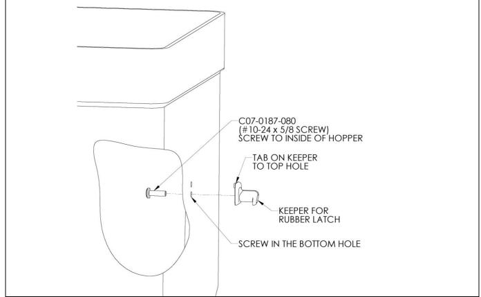
Assemble rubber latch keeper to the two holes on the side of the poly hopper using one  $\#10-24 \times 5/8$  screw (C07-0187-080) as shown. Repeat for the second keeper on the other side of hopper.
