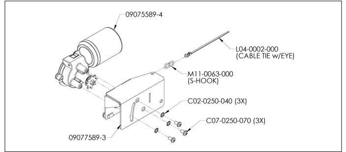
12-Volt electric motor wiring: Red (+) / Black (-). (NOTE: Screws & Shake Proof Washers are a part of electric motor.)
