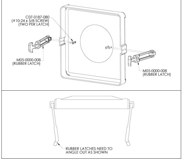
Assemble both rubber latches to the two holes on the side of the poly hopper cover using the  $\#10-24 \times 5/8$  screws (C07-0187-080) as shown.
