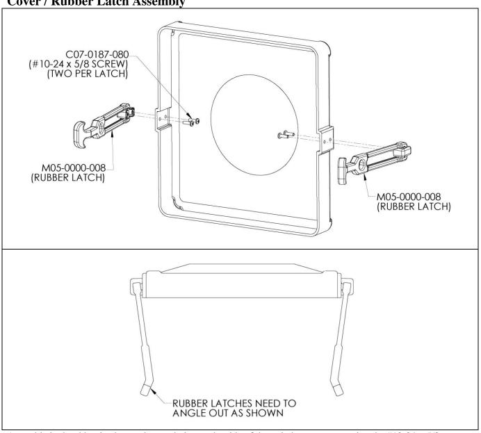
Assemble both rubber latches to the two holes on the side of the poly hopper cover using the #10-24 x 5/8 screws (C07-0187-080) as shown.
