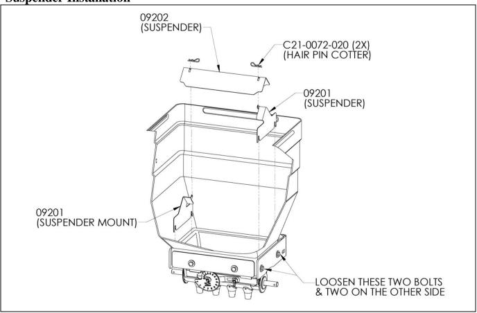
Loosen the bolts shown in diagram above. Locate suspender mounts (09201) and push insert mount down between hopper and bottom insert (silver in color) until it bottoms out on the two bolts that were loosened. Repeat for other mount. Tighten the two bolts on each side securely. Place suspender plate (09202) on top of the mounts. Secure in place using the two hair pin cotters supplied in the hardware bag.
