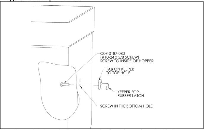
Assemble rubber latch keeper to the two holes on the side of the poly hopper using one  $#10-24 \times 5/8$  screw (C07-0187-080) as shown. Repeat for the second keeper on the other side of hopper.
