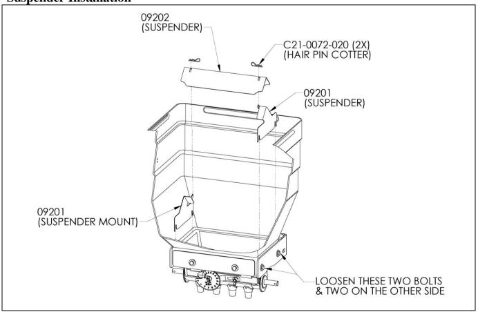
Loosen the bolts shown in diagram above. Locate suspender mounts (09201) and push insert mount down between hopper and bottom insert (silver in color) until it bottoms out on the two bolts that were loosened. Repeat for other mount. Tighten the two bolts on each side securely. Place suspender plate (09202) on top of the mounts. Secure in place using the two hair pin cotters supplied in the hardware bag.
