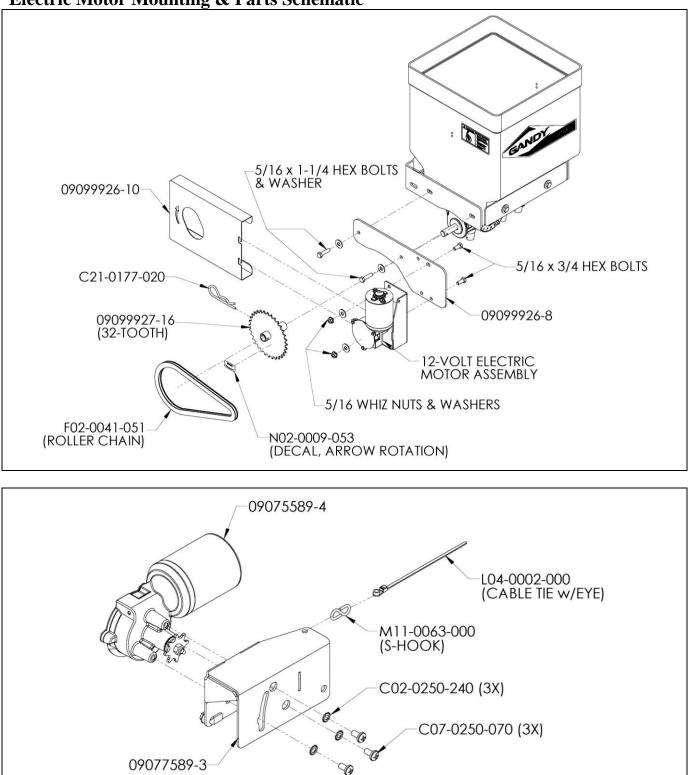
12-Volt electric motor wiring: Green (+) / Black (-). (NOTE: Screws & Shake Proof Washers are a part of electric motor.)
