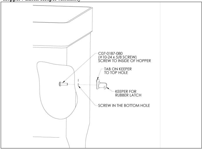
Assemble rubber latch keeper to the two holes on the side of the poly hopper using one  $\#10-24 \times 5/8$  screw (C07-0187-080) as shown. Repeat for the second keeper on the other side of hopper.
