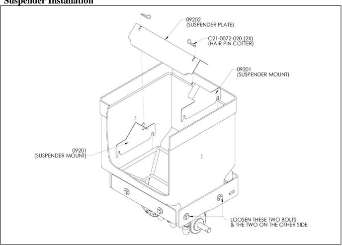
Loosen the bolts shown in diagram above. Locate suspender mounts (09201) and push insert mount down between hopper and bottom insert (silver in color) until it bottoms out on the two bolts that were loosened. Repeat for other mount. Tighten the two bolts on each side securely. Place suspender plate (09202) on top of the mounts. Secure in place using the two hair pin cotters supplied in the hardware bag.
