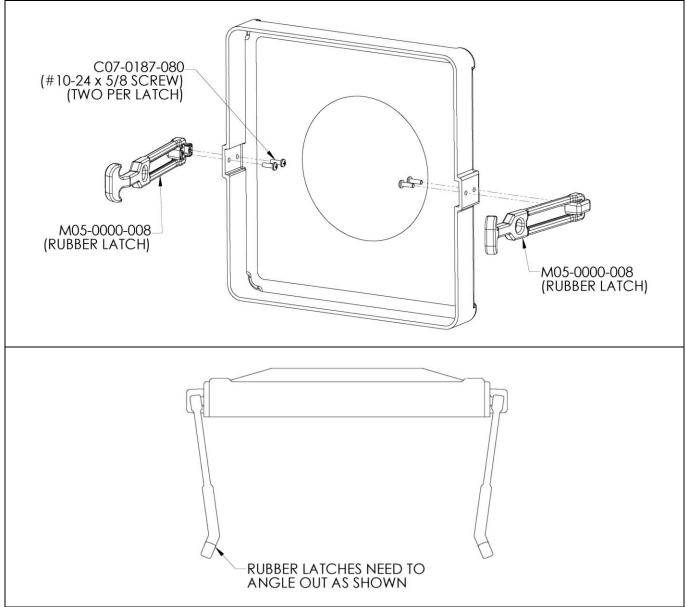
Assemble both rubber latches to the two holes on the side of the poly hopper cover using the  $#10-24 \times 5/8$  screws (C07-0187-080) as shown.
