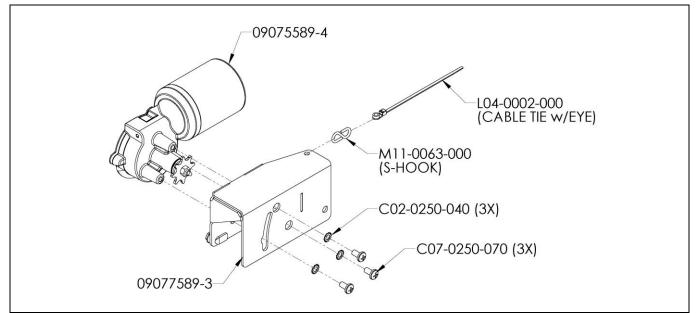
12-Volt electric motor wiring: Green (+) / Black (-). (NOTE: Screws & Shake Proof Washers are a part of electric motor.)
