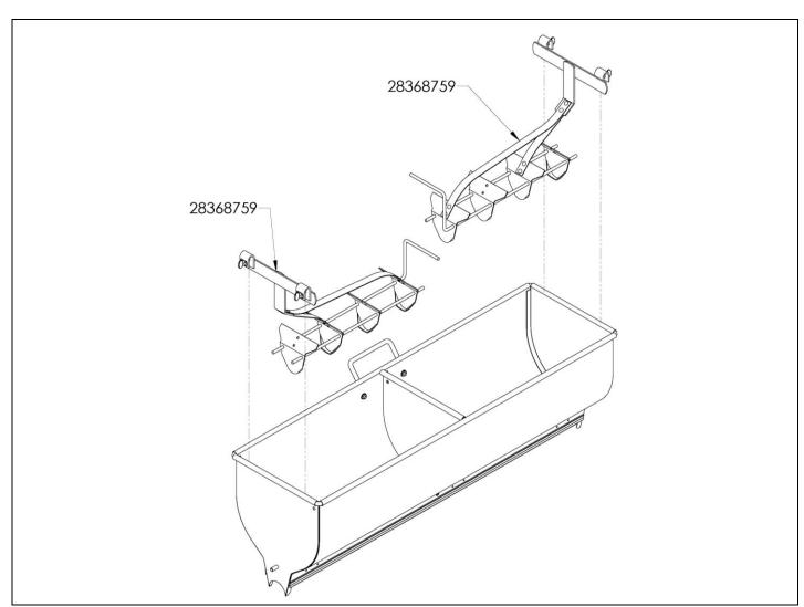
Attach Jigglers (one each side) over the outside round edge and tighten the thumb screws.
