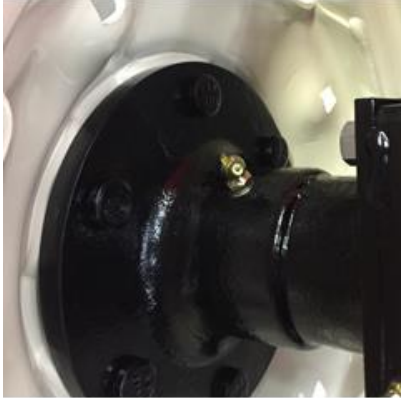
One Grease Fitting on Left & Right Wheel Hub
